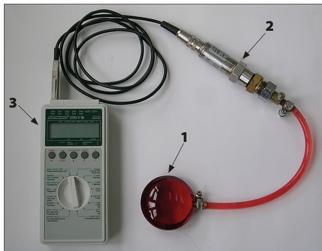
Figure 1. Hydro-electronic force meter and its components: 1 – Active Liquid Pad (ALP); 2 – pressure transducer; 3 – electronic manometer
